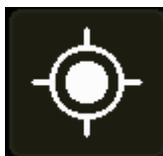
The GPS button will flash if the last GPS fix is more than 24hrs old and a fix is required for the recording mode. It will also change to a Transect icon
