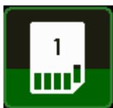
The SD Card buttons indicate the amount of used space with a colour fill. If the colour is green you still have more than 50% free space, orange indicates 50 – 90% of your card is used, and red indicates you have less than 10% remaining. If there is no SD card inserted, the icon will be greyed out and flashing to indicate an issue. If you press on an SD Card button you will enter the [SD Card Menu](#).
