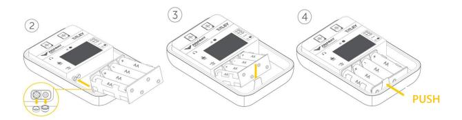
IMPORTANT: Do not allow the battery holder terminals to short out against metal objects. Always remove the batteries from the holder as soon as it is disconnected from the Swift. Do not store batteries in the holder.
